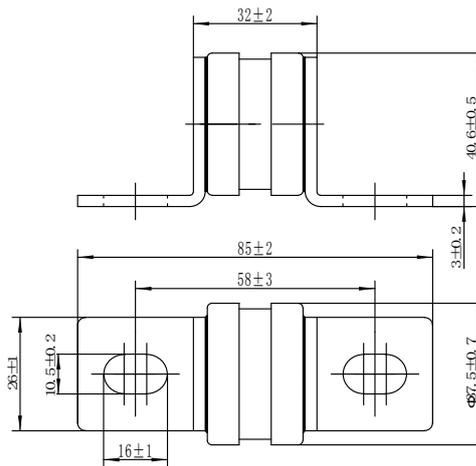
3NM-熔断件外形及安装尺寸
