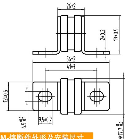
3NL-熔断件外形及安装尺寸
