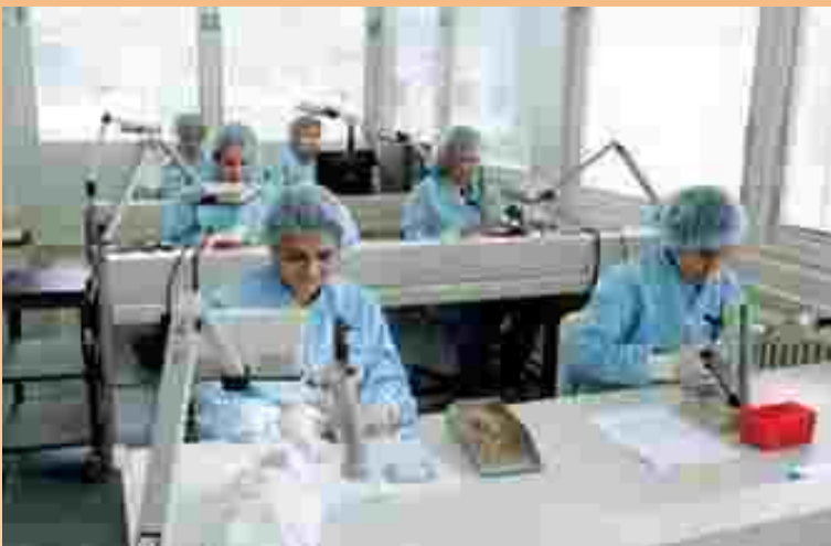
Clean room, assembly of fibre optic contacts
